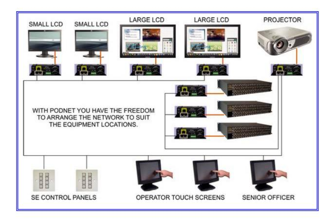
Here it is a simple matter of assigning network messages to each control panel and programming each control processor with the messages it needs to respond to. As each processor received messages directly, via the network, from any and all control panels assigned to it, any network delays are reduced and even in the event of a panel failing, the others will still operate the controllers. We now have our ninth guideline in designing critical systems: -
