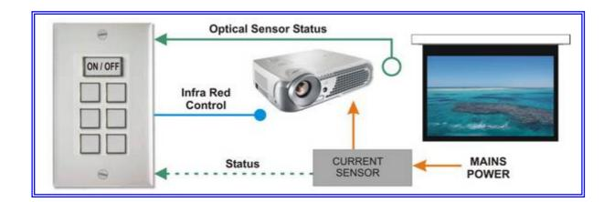
With systems that only transmit RS232 it's the same story so it always best to use a bi-directional RS232 port and configure the system to interrogate the display as to its status and communicate accordingly to ensure its not only on but ready for use.
