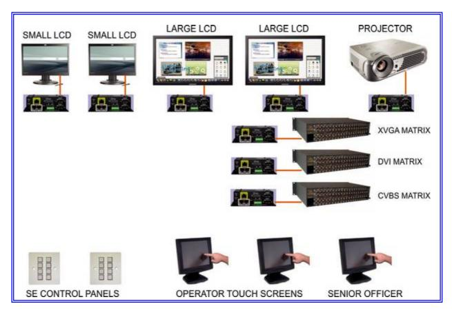
What we have here is for each matrix and each display we have a dedicated control interface. These each communicate with the matrix or display via RS232 and are configured to carry out the handshaking of commands we discussed right back at the beginning with the projector control example. Having assigned this level of 'housekeeping' to each controller we can minimise network traffic required for this important function.
