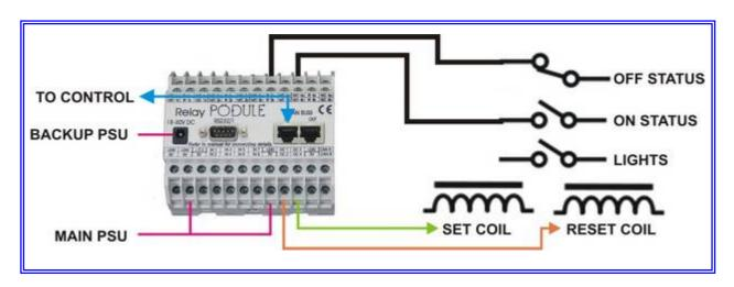
The Relay Podule from iKON AVS is a self-contained controller with internal power relays and its own processor and whilst it will operate in isolation, it is normally linked by a propriety network to control panels and other processors.
