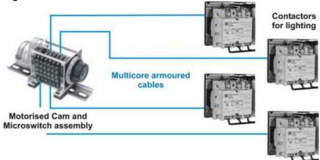
As the coils all operated at 24V, the original system used separate armoured multicore cables from the central control room to the remote plant rooms but over time these cables had deteriorated due to water ingress or had been damaged by building works.
