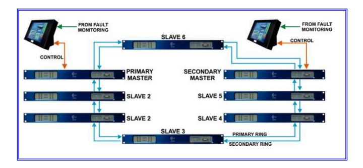
The above diagram shows a simplified version of the audio distribution system. The units selected use two independent fibre rings with both carrying audio and embedded control simultaneously. Each unit is configured to monitor the unit preceding it on both primary and secondary circuits and report any network faults to an independent fault monitoring network.
