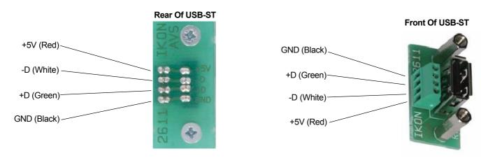
New version has a 5 way screw terminal S-GND to be used for the shield / braiding of the cable
