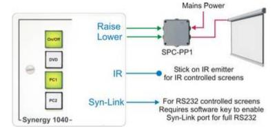
You can use external 12V DC relays for the power control as an alternative to the SPC-PP1, please see 'Alternative use of outputs' on the next page for details.
