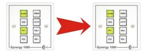
Operations on the slave panel only control devices connected to the slave panel while operations on the master panel control both its controlled devices as well as the ones connected to the slave. The buttons on the slave panel reflect the current status in both modes of operation. The panel linking can be enabled and disabled using the auxiliary inputs on the master panel, (e.g. from a room divide sensor).
