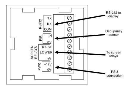
RS232 Tx, Com and the two Pwr connections MUST be used, the others are optional depending on your system Requirements!
