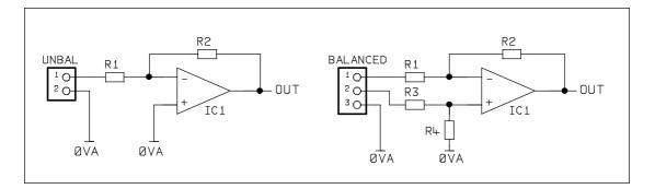
Looking first at the balanced input, here we treat the phase and anti-phase signals quite correctly as the send and return ensuring that both are routed to the active device as directly as possible and with minimum track length. The ground connection here is not part of the signal, it only provided RF and EMC screening, so it can quite safely be connected direct to any ground plane to return any induced currents to the reference ground and not the input circuit.
