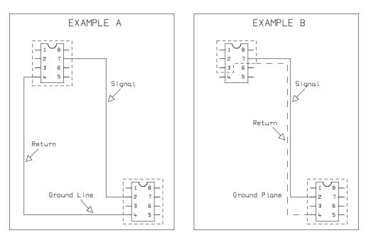
**Example A** is a bad design. It does not utilise an analogue ground plane at all. A loop is formed by the ground and signal traces.
