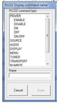
7. In the main control window double click on the white box and a window will open allowing you to add the RS232 command
