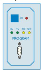
The Rx and Tx leds flash to confirm fibre communications.
