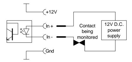
The Opto-diodes can be driven by active outputs as shown below
