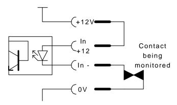
Using an external power supply.
