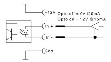
**N.B.** If an external supply or active drive is used, careful attention must be taken over ground routing.
