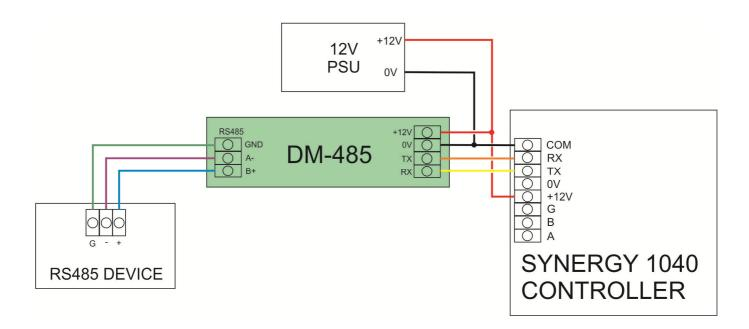
The power supply needs to be between 12V and 30V DC.
